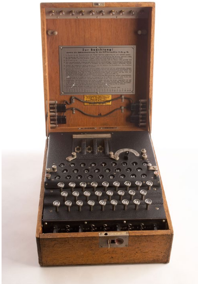
Figure 2-3. The Enigma machine (Source: Central Intelligence Agency)
